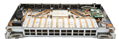
FIGURE 6. HPE Slingshot switch blade
