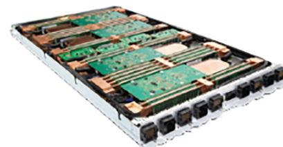
FIGURE 5. HPE Cray EX425 compute blade
